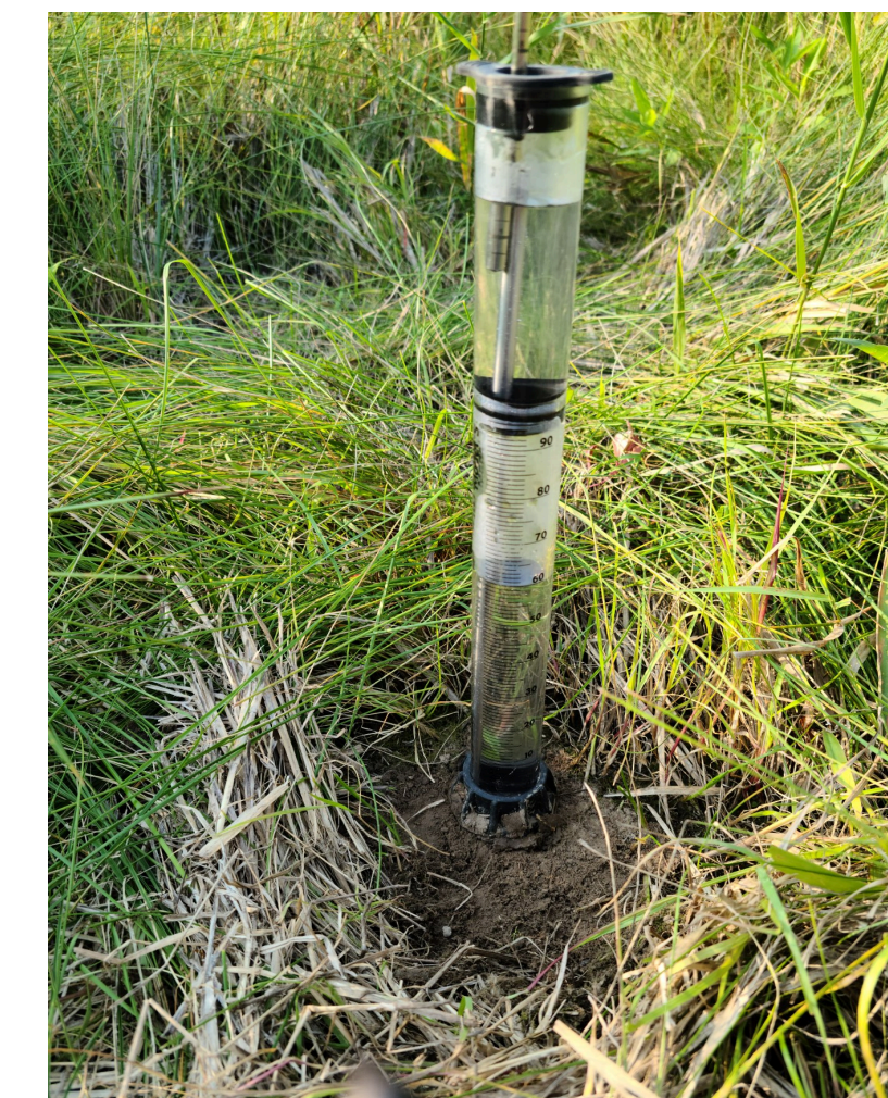
Figure 5. Mini Disk Tension Infiltrrometer placed on bare earth with measurements recorded every 30 seconds for 5 minutes.
