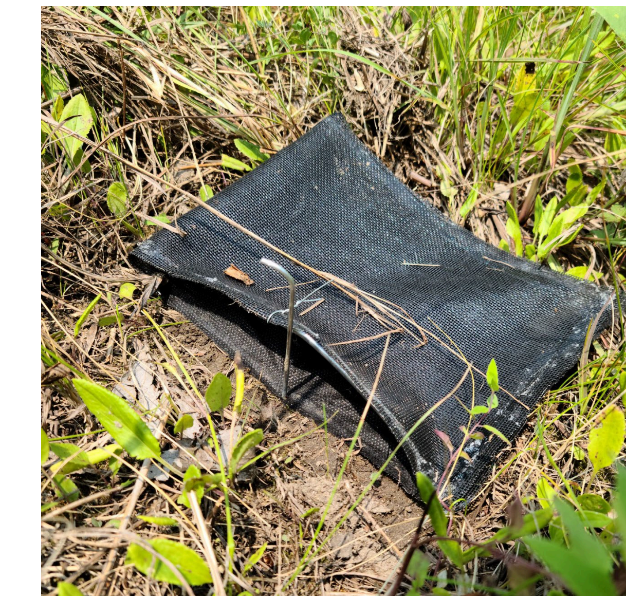
Figure 10. One of 45 sediment runoff traps constructed and set-up on remnant, restored, and impaired prairie.
